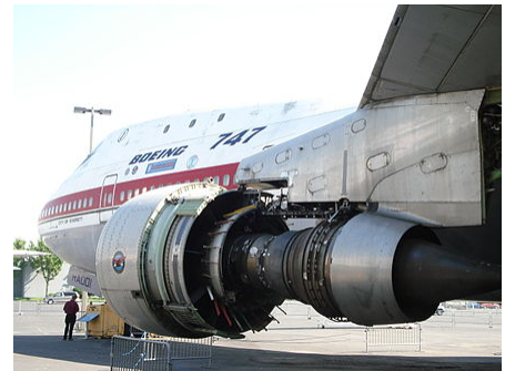
A JT9D turbofan jet engine installed on a Boeing 747 aircraft.
